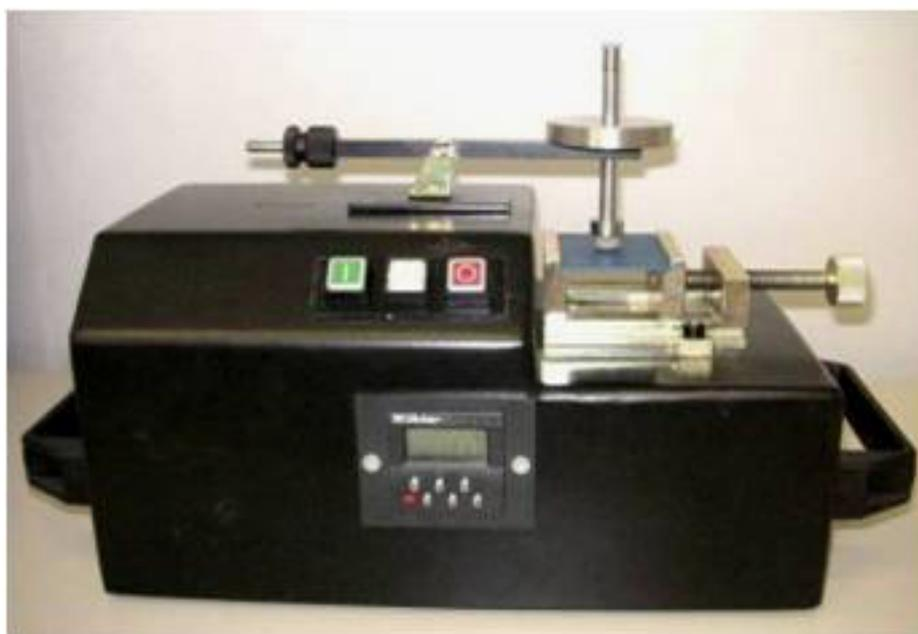
Fig. 2. Stroke tester for wipe testing
