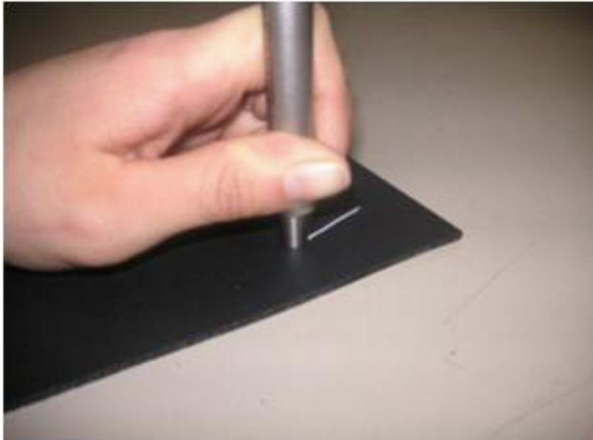
Fig. 3: hardness pen for scratch testing
